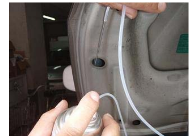
Anti-rust coating under hood
