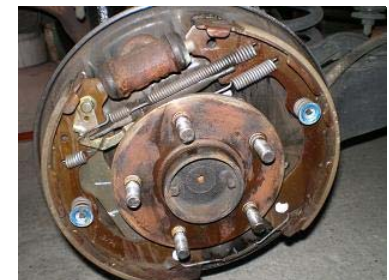
Maintenance for drum break
