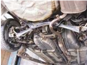
Loosen rust bolts & nuts for exhaust pipe.
