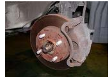
Maintenance for disk break
