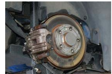
Maintenance for disk break
