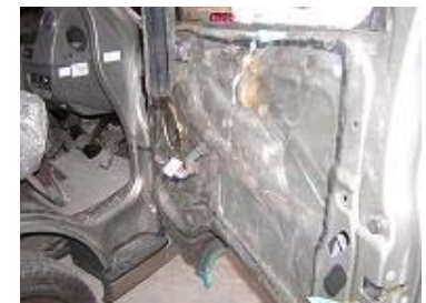
Anti-rust coating for inside door
