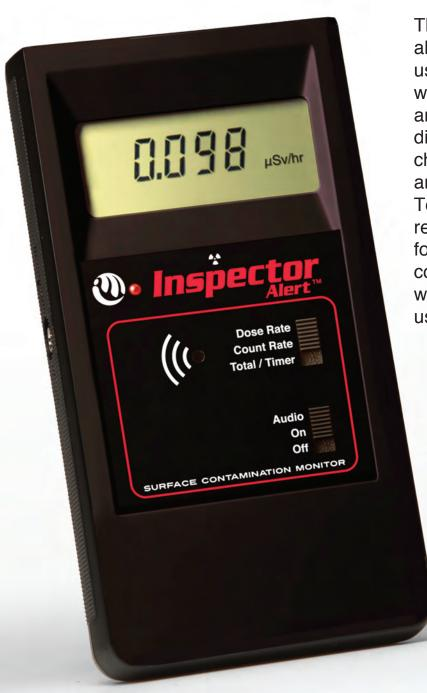
The IMI Inspector Alert™ V2 measures alpha, beta, gamma and X-radiation using a 2-inch "pancake" GM detector with high sensitivity to common beta and alpha sources. The easy-to-read digital display shows reading in your choice of Dose Rate - µSv/hr or mR/hr, and Count Rate - CPM or CPS. The Total / Timer feature allows timed readings from one minute to 40 hours for precise measurement of low-level contamination. An Audible alert sounds when the radiation reaches a user-adjustable level.
