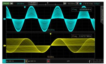
Signals with different clock sources and large frequency difference can also display the waveform stably on the screen, which is convenient for customers to analyze the waveform parameters.
