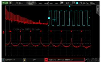
UP01000CS series has 1 M FFT sampling points. It can also set the practical functions of spectrum analyzer such as frequency range, detection mode and spectrum marking. It is convenient for you to analyze the signal in frequency domain on oscilloscope.
