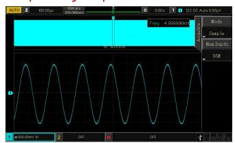
UPO1000CS series 56M sampling points per channel. This enables the oscilloscope to maintain high sampling rate in a wider time base range, At the same time considering the whole and details of the waveform, which greatly improves the ability to capture abnormal waveforms.
