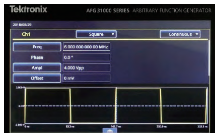
With InstaView on AFG31000 turned off. Due to an impedance mismatch, the AFG display shows a different waveform from the one observed at the DUT.
