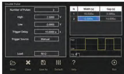
AFG31000 Double Pulse user interface
