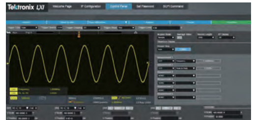
Built-in web page enables remote control of horizontal and vertical scale, trigger settings, and measurements.
