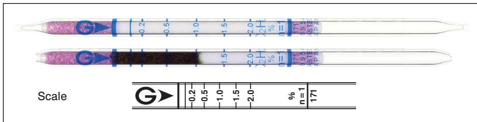
**Performance** The minimum scale value (0.1%) is not printed on the tube, but only the scale line is printed.
