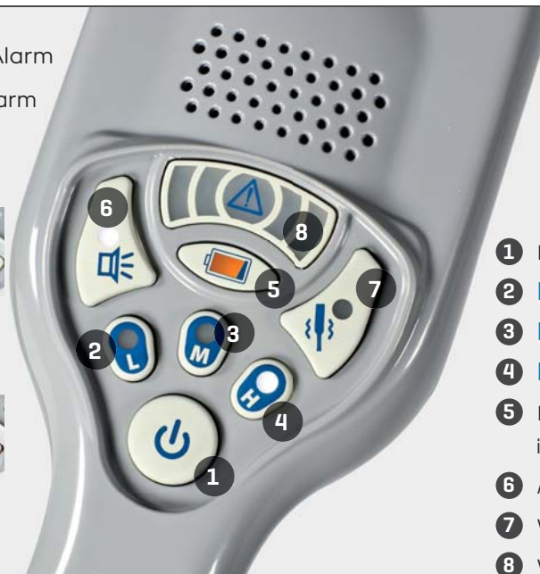
Optical indication proportional to the metal signal strength [Low, Medium, High].
