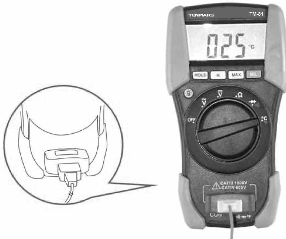
Fig. 7: Using the instrument for Temperature measurement
