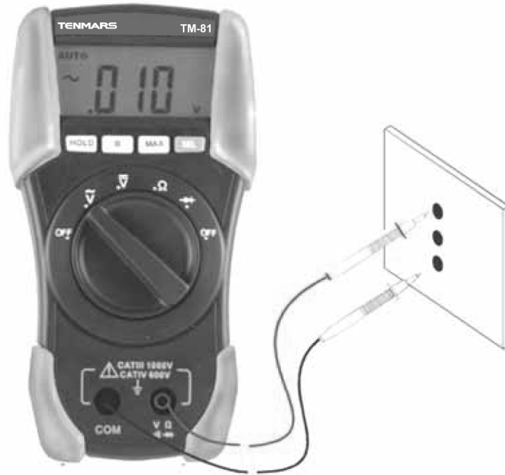
Fig. 3: Using the instrument for AC Voltage measurement
