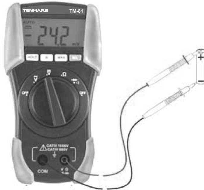
Fig. 2: Using the meter for DC Voltage measurement
