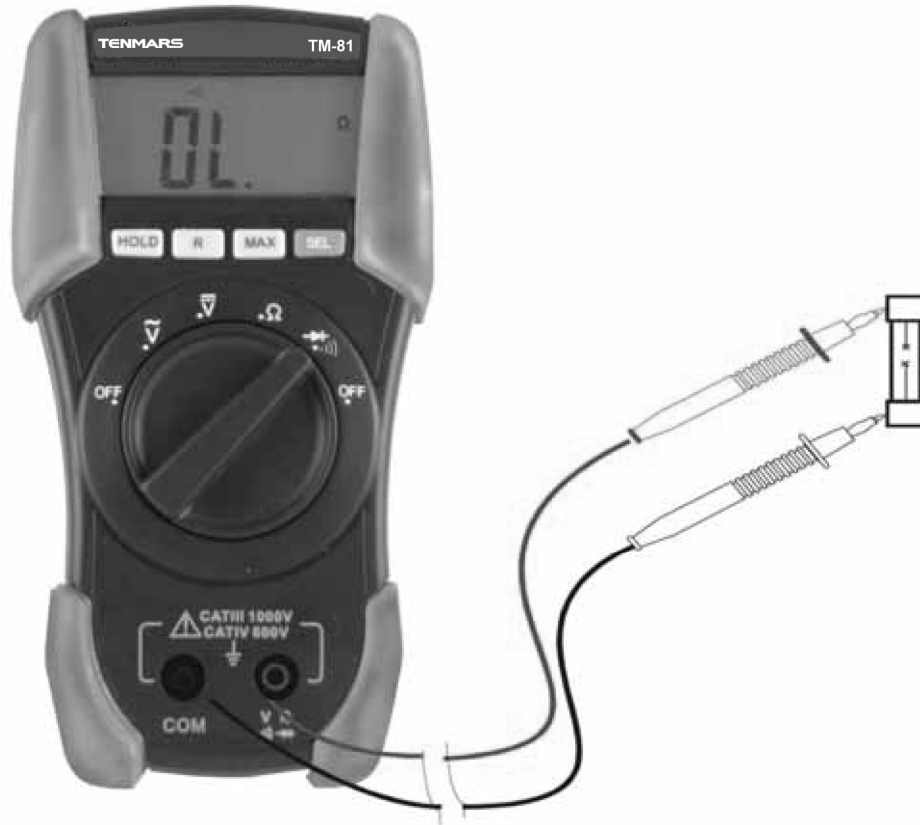
Fig. 5: Using the instrument for continuity test
