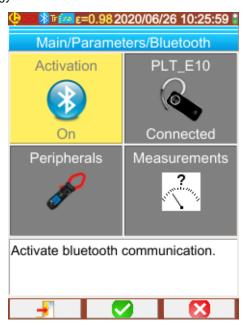
To use this function, you must first activate it from the Main/Parameters/Bluetooth menu by setting the Activation
