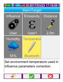
In case of Influence parameters, the measurements replace the user data entered in the Main/Target menu, provided that user influence is selected (see §3.2. Use influencing parameters consistent with the conditions of measurement).
