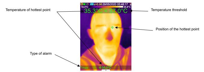
When making your measurements, take care not to have of heat source other than the subject in the field of view of the camera, and make sure that the hot spot is in fact on the desired target, since otherwise you risk triggering the alarm as shown below:
