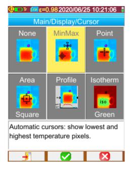
By default, it is the MinMax cursor that is selected in the Main/Display/Cursor menu, and the camera produces only infrared images.
