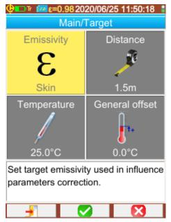
The emissivity is the most decisive of the adjustments for the measurement of body temperatures. It is set to that of skin (0.98).
