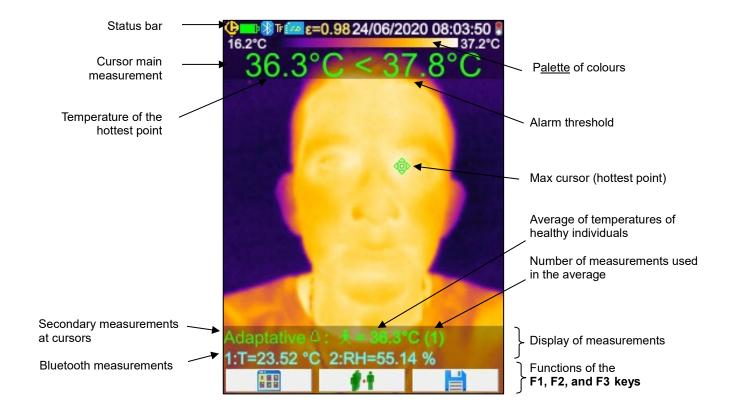
The ~ symbol before the reading indicates that the camera has not yet stabilized.
