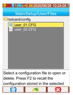
A setup file is recalled from the Main/Setup/User/Files menu, by means of the file manager, which lists all of the configuration files (extension .CFG) found in directory « /media/sdcard/config/ ».
