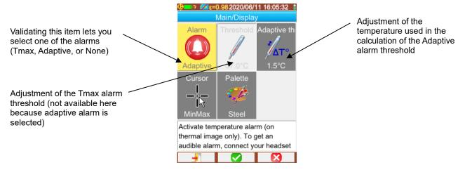
The activation of an alarm forces display of the **MinMax cursor** used to display the measurements, the max cursor indicates at each acquisition the position of the highest temperature; the measurement displayed is stabilized for better reading comfort and to limit spurious triggering.
