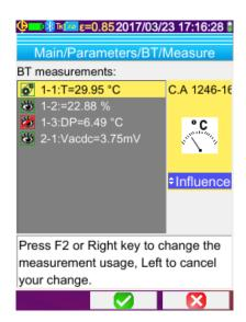
For the measurement to be used as an **influence**, the use "influence" must be assigned to it in the Bluetooth measurements viewing window (Main/Parameters/Bluetooth/Measurements menu):
