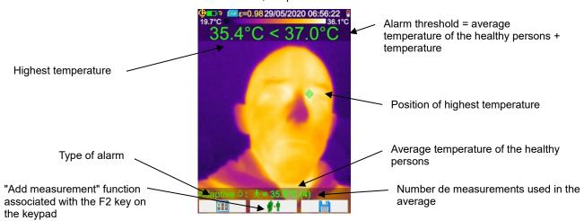
A measurement is selected by pressing the function key Fx associated with the function or by pressing the trigger, when the TL ("Load measurement") function is selected (see §1.5.4. Changing the function associated with the trigger of the camera).
